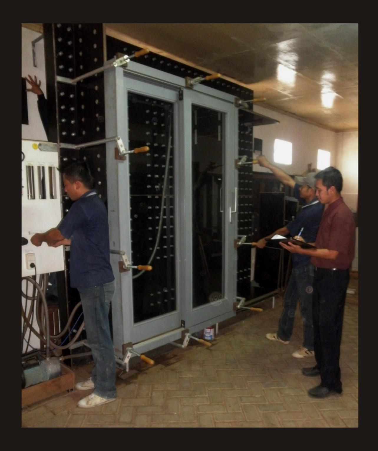
Because much of Sarana's output is destined for the tropical beaches of The Pacific and Caribbean Islands, Sarana has its own testing facilities to monitor the wind and water performance of the doors and windows. The company is licensed by Warnock Hersey to produce fire rated doors both single and double for periods up to 90 minutes
